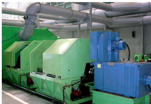
Fig. 4 brake performance dynamometer for high speed train
